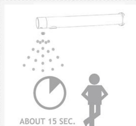
4. Turn on the central water supply. Check for leaks.
